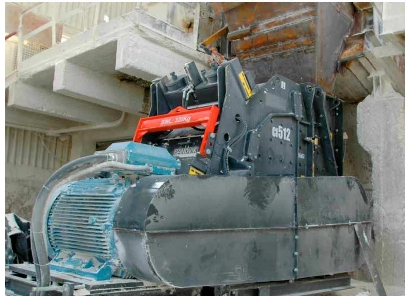
CI512 Secondary Crusher
