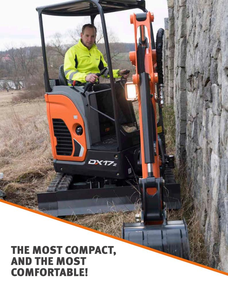
The sophisticated ISO-certified TOPS/ROPS/FOPS canopy – together with excellent visibility and stability – provide optimal operator comfort and safety. Comfortably seated, you have easy access to several storage compartments and a clear all-round view of the worksite. Noise and vibration levels are minimised.
