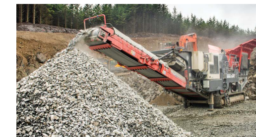
Extended main conveyor for massive stockpiling
