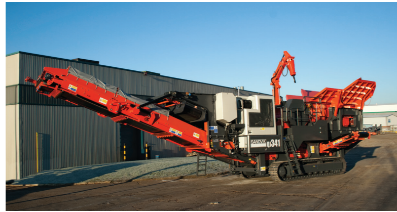
Optional hydraulic breaker arm with hammer and hopper extensions available
