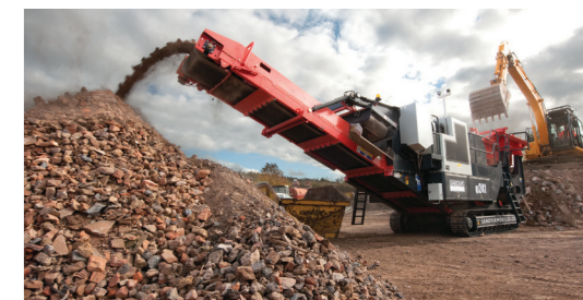
Extended main conveyor for massive stockpiling
