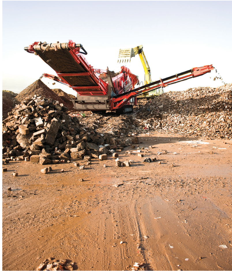
Ability to configure with punch plate, grizzly fingers, bofar bars, mesh or cascade fingers
