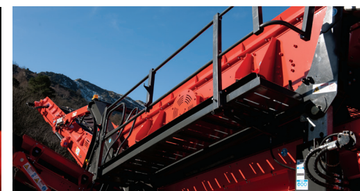
Hydraulically folding maintenance platforms
