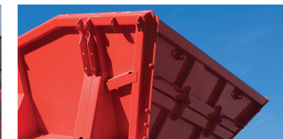
Split rear hopper door for direct feeding
