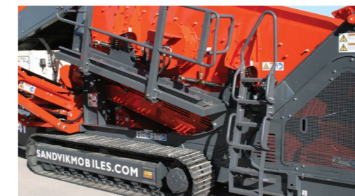
Incline ladders for screenbox access
