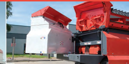
Hydraulically opening powerpack for ease of maintenance
