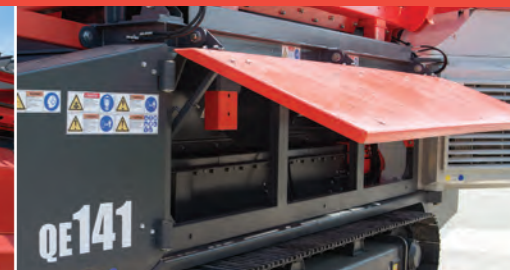
Hydraulically folding doors for easy access
