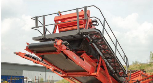
Three sided walkway around main conveyor
