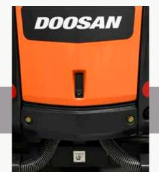
Lockable cap: Unique & safe access point for all maintenance checks.
